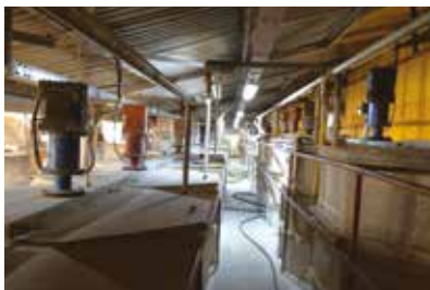
Glazur Mixer - 185 Nm - 30 rpm
